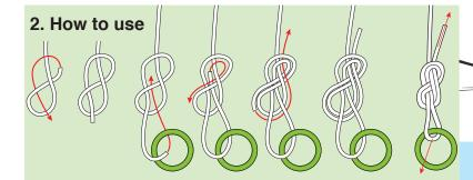
The aluminium ring needs to be entered into the setup while installing the highline. Both, main and backup line must be threaded through the ring. Prior to that, the leash ring must be connected to the leash rope with a figure-8-knot (see drawing)
