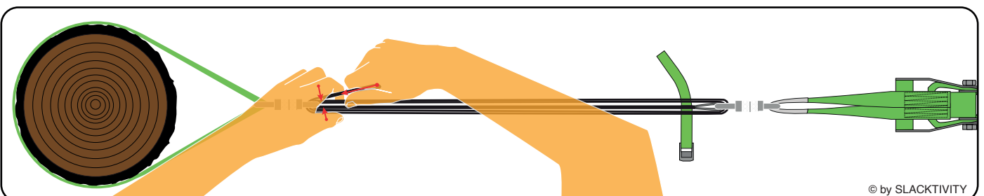
The releasing speed can be controlled by squeezing the softRelease together by hand and feeding the webbing through.
